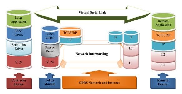
This particular implementation allows to the devices interfacing to the Telit GE910 module the use of the GPRS and Internet packet service without the need to have an internal TCP/IP stack since this function is embedded in the module.
